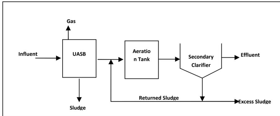
**Schematic Diagram of an Upflow Anaerobic Sludge Blanket Process followed by ASP**
