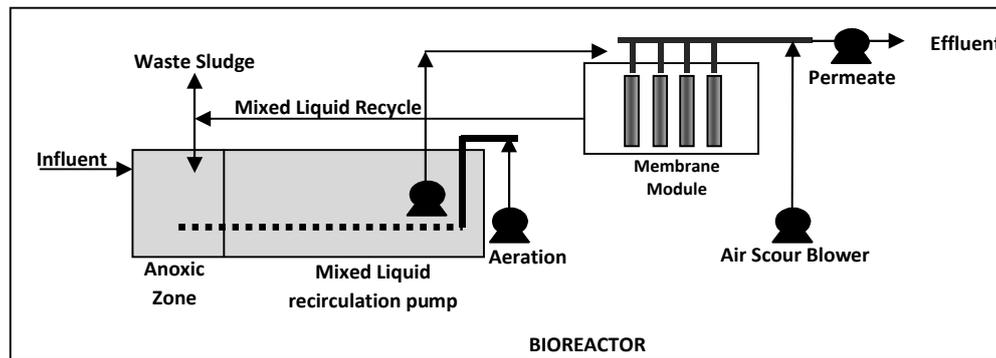
**Schematic Diagram of a Membrane Bioreactor**
