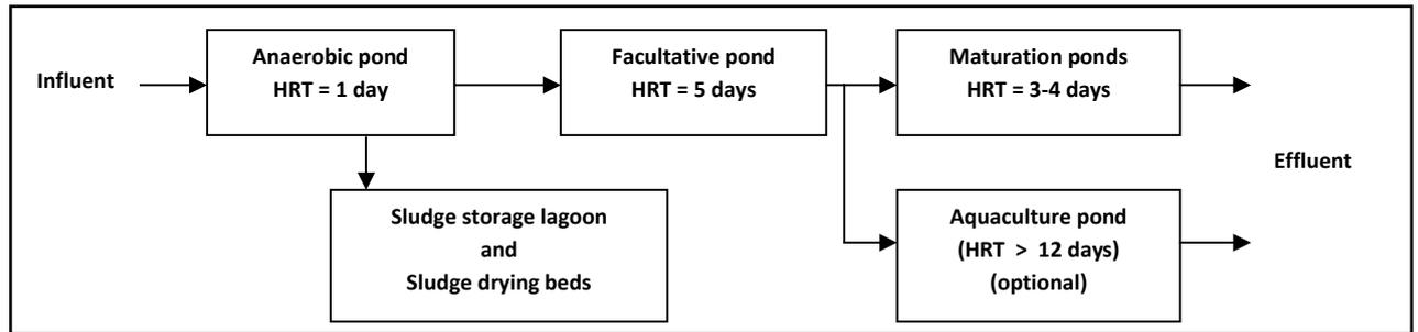
**Schematic Diagram of a Waste Stabilization Pond**
