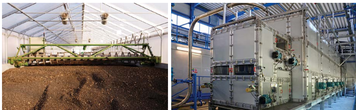
Figure 7: Solar drying in greenhouses (left) and thermal dryer (right). Credit photo: suzewatertechnologies.com
