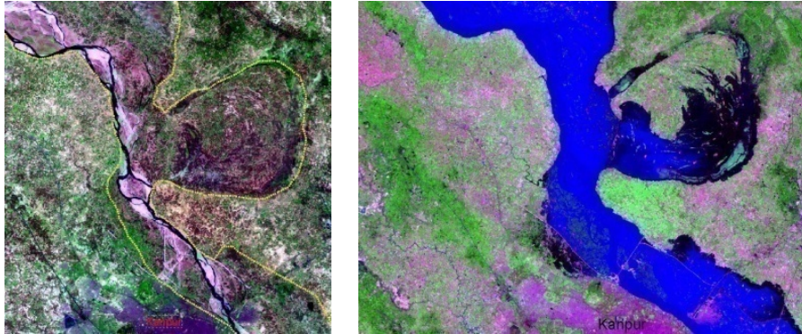
Figure 1: (a) LANDSAT 2003 data showing the meander scroll and the stretch of Ganga upstream of Kanpur. The active floodplain of the river is shown with a dashed line. Note that the right bank of the river does not have any active floodplain whereas the left bank has a wide floodplain. (b) LANDSAT data of the Kanpur area during the flood of 2010.
