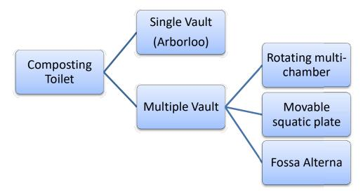
Figure 3.4 Classification of Composting Toilets, according to GTZ, 2010 [15]
