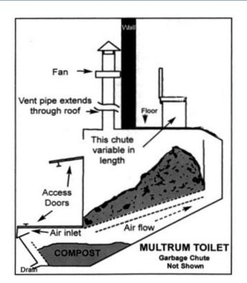
Figure 3.3 General schematic diagram of a Composting Toilet Source: Adapted from the Humanure Handbook To increase composting properties, dry material, such as sawdust or ash are added. This regulates the carbon to nitrogen ratio (C/N) and enhances the composting process. If ash and lime are used as bulking material, there is the additional beneficial effect of raising pH, which leads to improved pathogen die-off [14].
