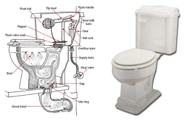
Figure 3.8: Design of a Flush Toilet, Source EAWAG/SANDEC, 2008 [13]
