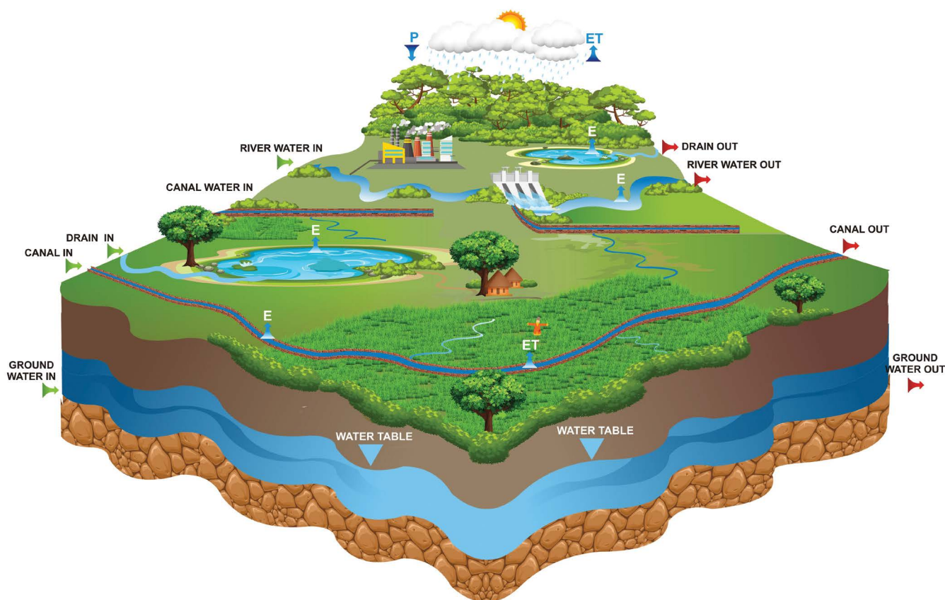
Figure 4: Depiction of various components to carry out water balance in a geographical area
