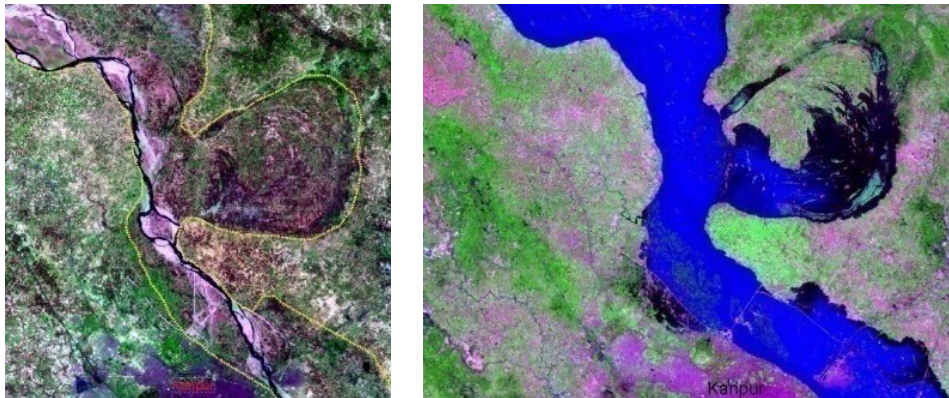
Figure 1: (a) LANDSAT 2003 data showing the meander scroll and the stretch of Ganga upstream of Kanpur. The active floodplain of the river is shown with a dashed line. Note that the right bank of the river does not have any active floodplain whereas the left bank has a wide floodplain. (b) LANDSAT data of the Kanpur area during the flood of 2010.
