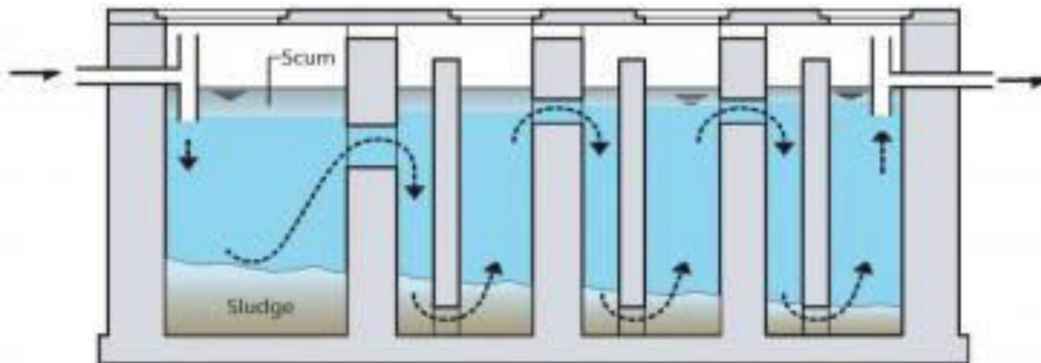
**Figure 4.2: Schematic cross-section of an Up-Flow Anaerobic Baffled Reactor**
