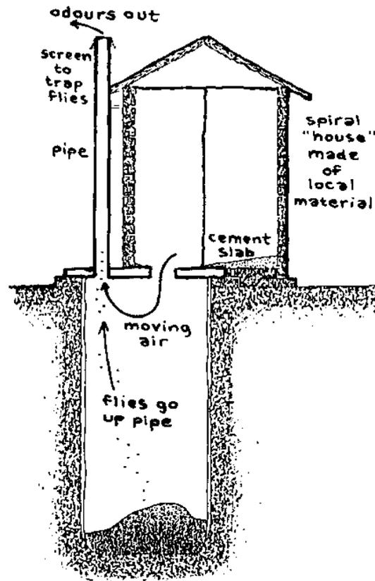
**Figure 3.2:** Schematic diagram of a Ventilated Improved Pit Latrine
