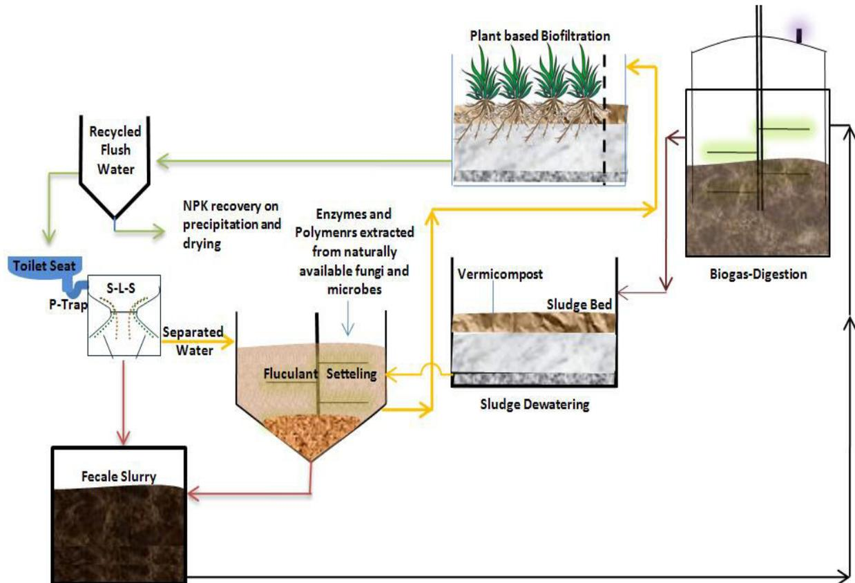
**Figure 3.10: Schematic diagram of Zero Discharge Toilet System**
