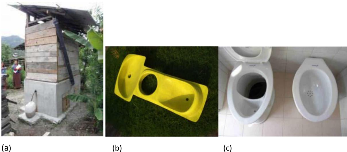
**Figure 3.7:** (a) Double-vault urine diversion dehydration toilet, Vietnamese style, Bhutan. Source: WAFLE (2009); (b) Urine-diversion squatting pan with anal cleansing water collection bowl (made from fibre-reinforced plastic). Source: WAFLE (2010); (c) Ceramic urine-diversion pedestal with separate bowl for collection of anal cleansing water. Source: UNESCO-IHE
