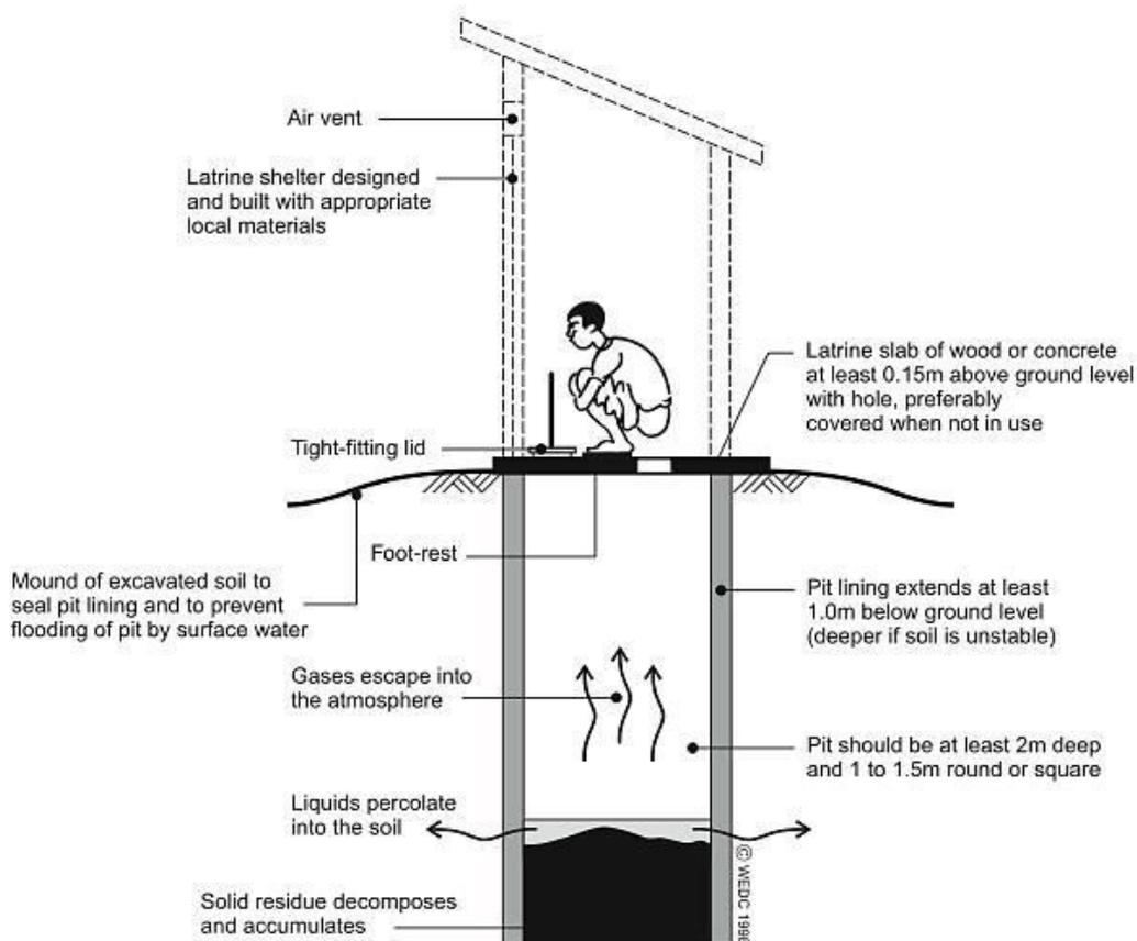
**Figure 3.1:** Schematic diagram of a simple pit latrine. Source: Harvey et al. 2002 [12]
