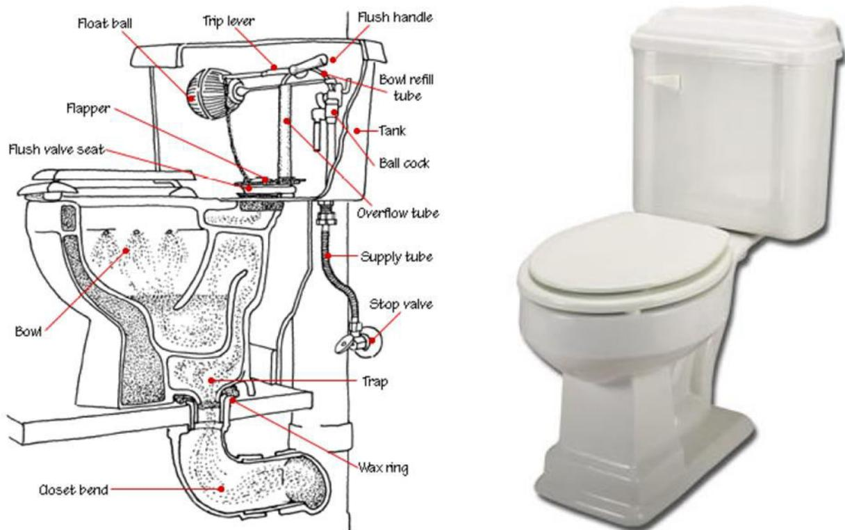
**Figure 3.8: Design of a Flush Toilet, Source EAWAG/SANDEC, 2008 [13]**
