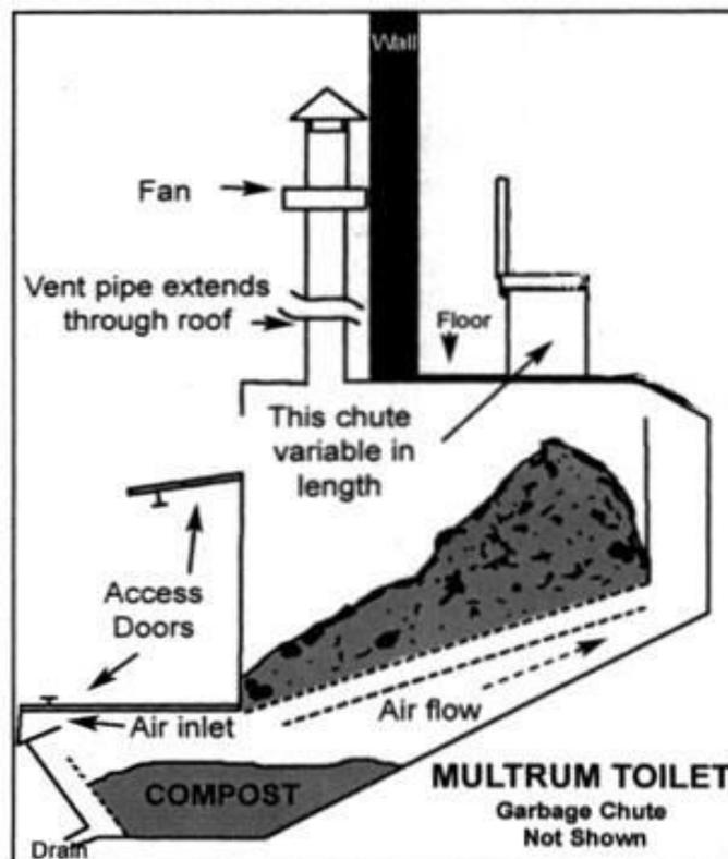
**Figure 3.3 General schematic diagram of a Composting Toilet**
